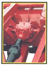
200 HP gearbox with overrunning clutch and constant velocity 1000 RPM PTO.
