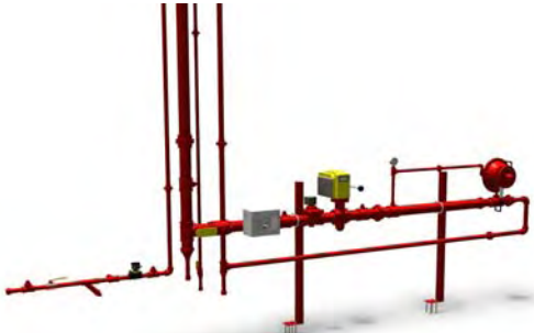
Figure 20: 12' Tower LPG Manifold"
