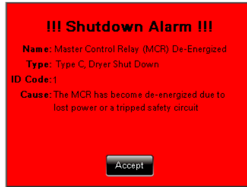
Figure 43: "Shutdown Alarm Pop up Screen"
