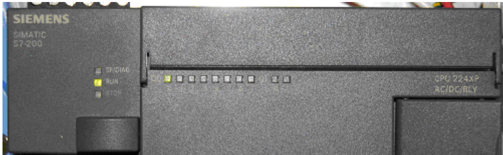
Figure 25: "Siemens PLC Module"
