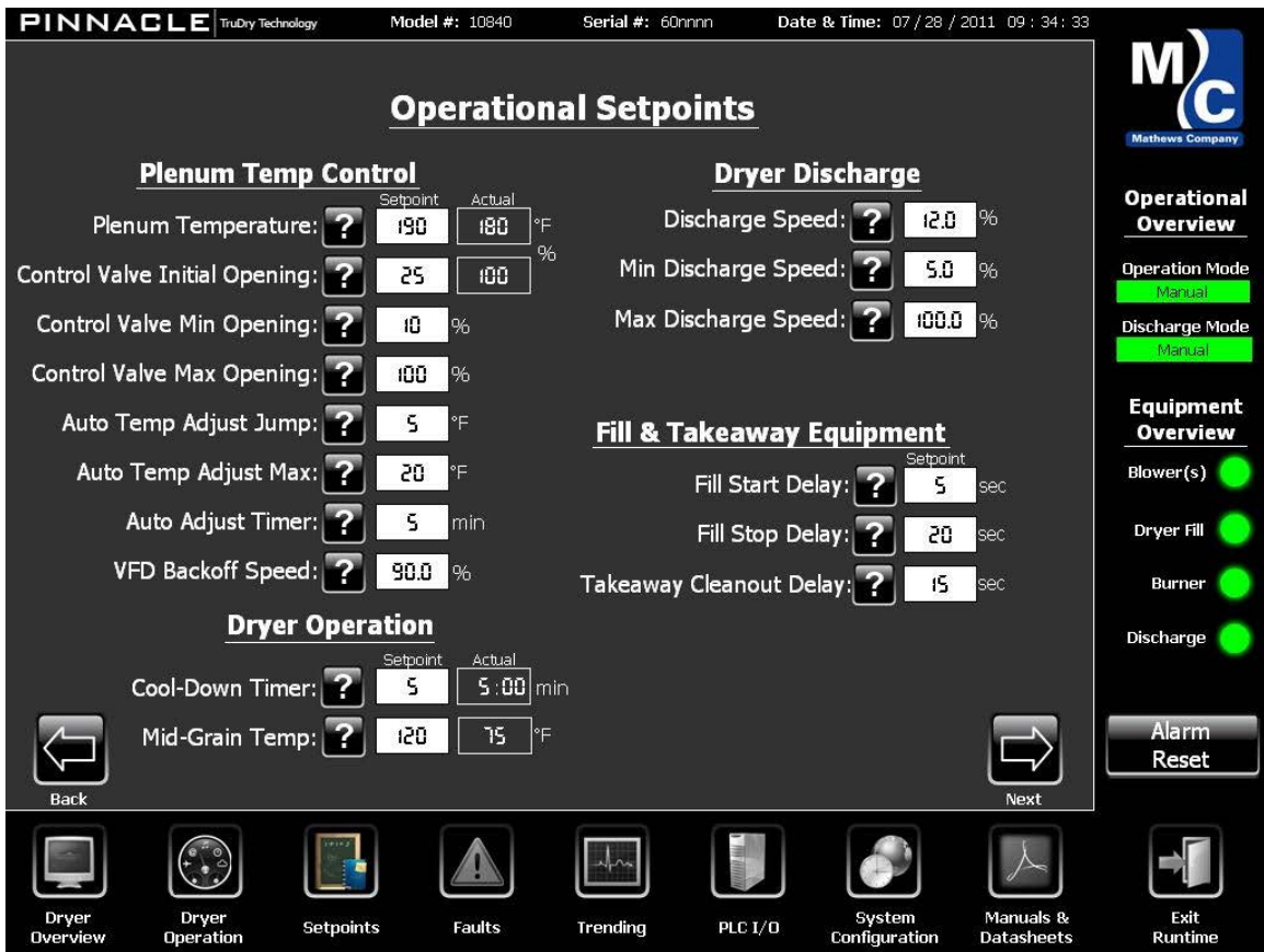
Figure 13: "Operational Set Point Screen"
