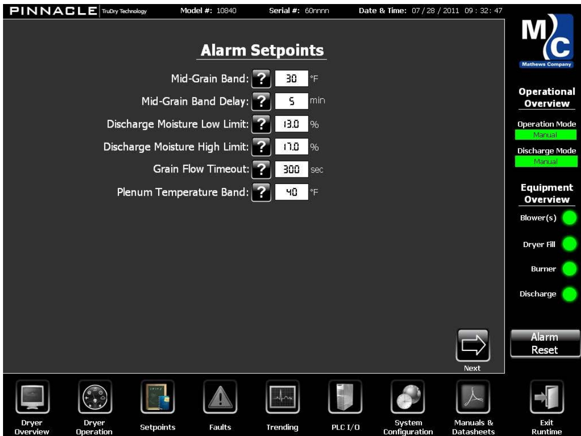
Figure 12: "Alarm Set Point Screen"
