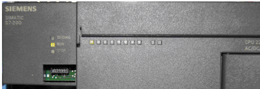
Figure 26: "Siemens PLC Module Chip Cover Removed"
