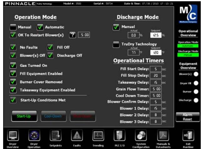
Figure 6: "Dryer Operation Screen AUTOMATIC Mode"
