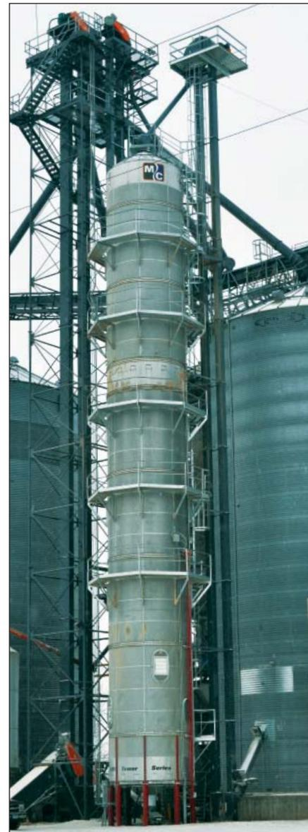
Propane-fired M-C 2,800-bph Model 12-28-150 tower dryer at Colfax Farmers Elevator Inc.
