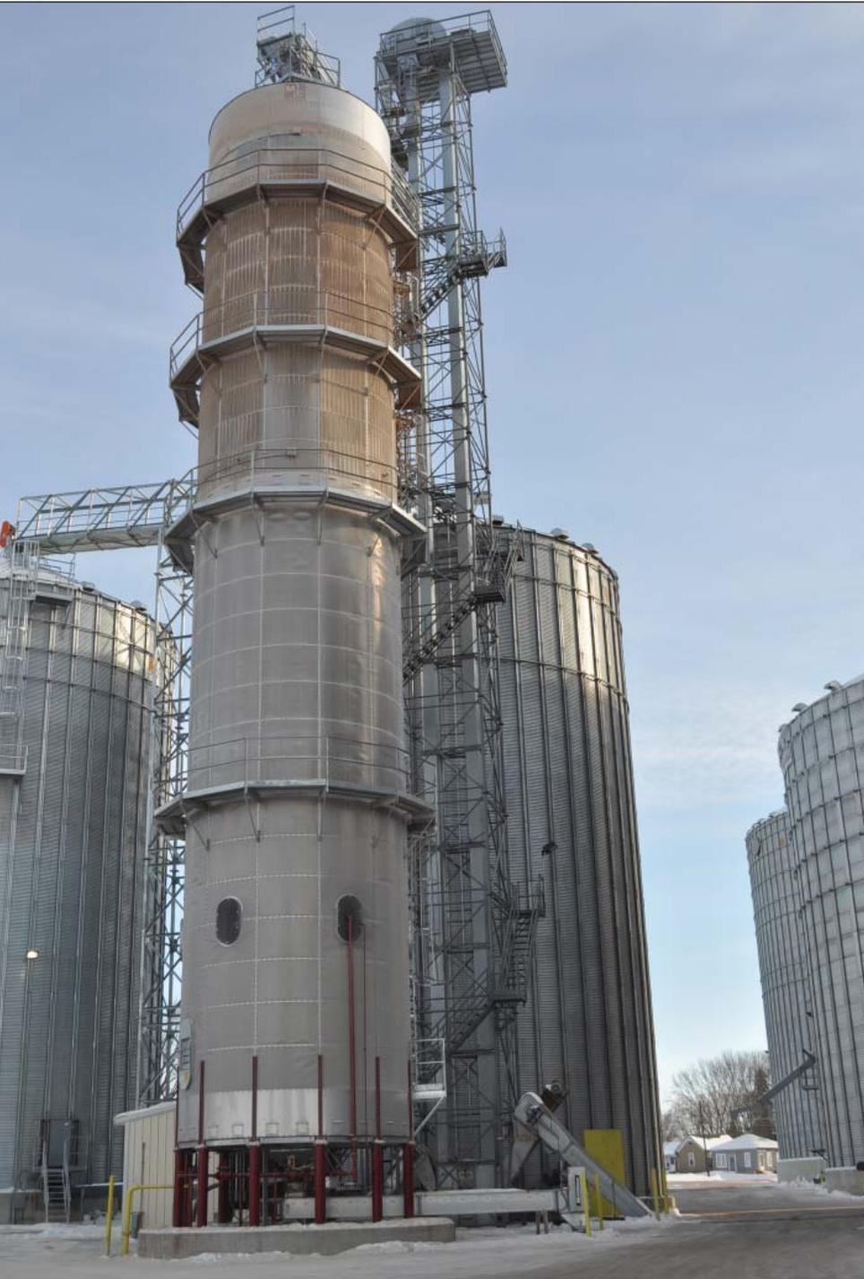
*M-C Model 4800 installed in 2012 at Northside Elevator Inc. in Loyal, WI rated at 4,800 bph at five points of moisture removal and the largest in Mathews Co.'s 18-foot series of tower dryers. Photo by Ed Zdrojewski.*
